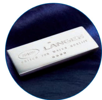
Fig. 5: Attractive waste! A silver bar made from recycled COD reagents.
